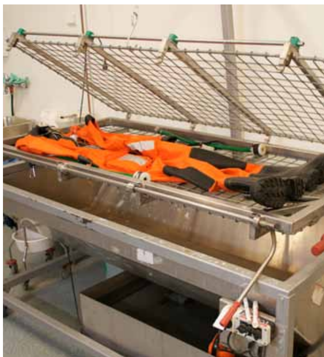
The drying cabinet is the most efficient way to prepare suits for delivery
